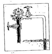
In this picture of an atmospheric vacuum breaker, a backsiphonage condition exists. This condition has caused the check-float to drop away from the air-inlet and seat on the check seat, which prevents the non-potable water from being backsiphoned. If the check-float did not seat properly, again only air would be sucked back into the domestic water system.
