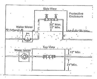
ssure Vacuum Breaker e pressure vacuum breaker. mot be installed where re can be backpressure. y where there can be ksiphonage. The pressure uum breaker can have. it-off valves downstream he device. The PVB must installed at least 12" above highest outlet or, if it is ding an open tank, at least above the highest irflow rim of the tank. The owing figure shows a cal installation on a nkler system.
